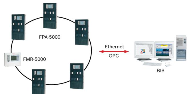
The FMR-5000 Remote Keypad offers the decentralized operation of a control panel or control panel network.
