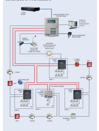
Loudspeakers, Loop DAU requires special 64 Ohm low impedance speakers Mains DAU uses standard 100v line speakers
